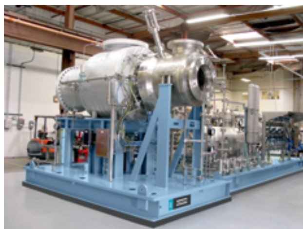
A turboexpander for cryogenic hydrocarbon separation.
